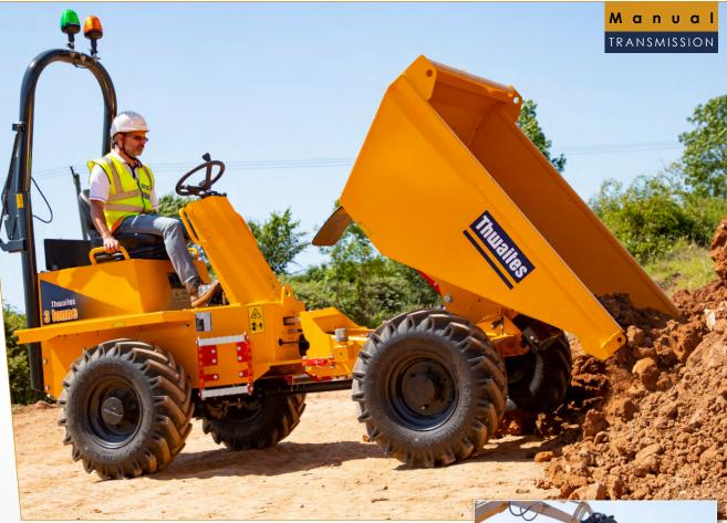
The Thwaites 3 Tonne Front Tip, Stage V dumper is manufactured with contractors and hirers in mind – ensuring operator safety, reducing risk on site and improving performance. Powered by an 18.1 kW Yanmar engine, delivering 107 Nm max torque for optimum traction and control. This machine is driven by a Manual transmission.
